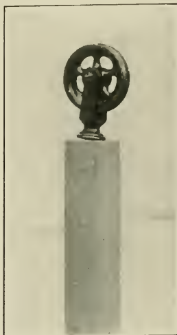
Fig. 390.—Pulley arranged on broom-handle to be fastened at foot of bed for carrying extension cord.
